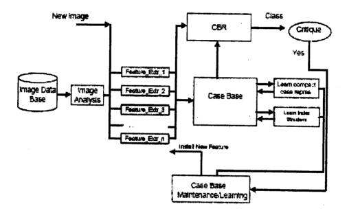
Figure 3: Architecture of the system.
