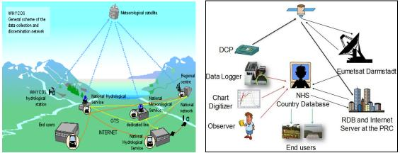
Figure 7: Satellite DCP Operation
