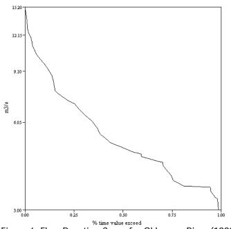
Figure 6: Flow Duration Curve for Okhuwan River (1990).
