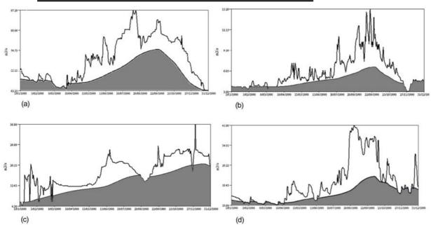
Figure 4: Hydrographs from the Ossiomo River Watershed in 1990: (a) Ossiomo at Ologbo (b) Okhuwan at Ugonoba (c) Ikpoba River at Benin City (d) Ossiomo at Abudu
