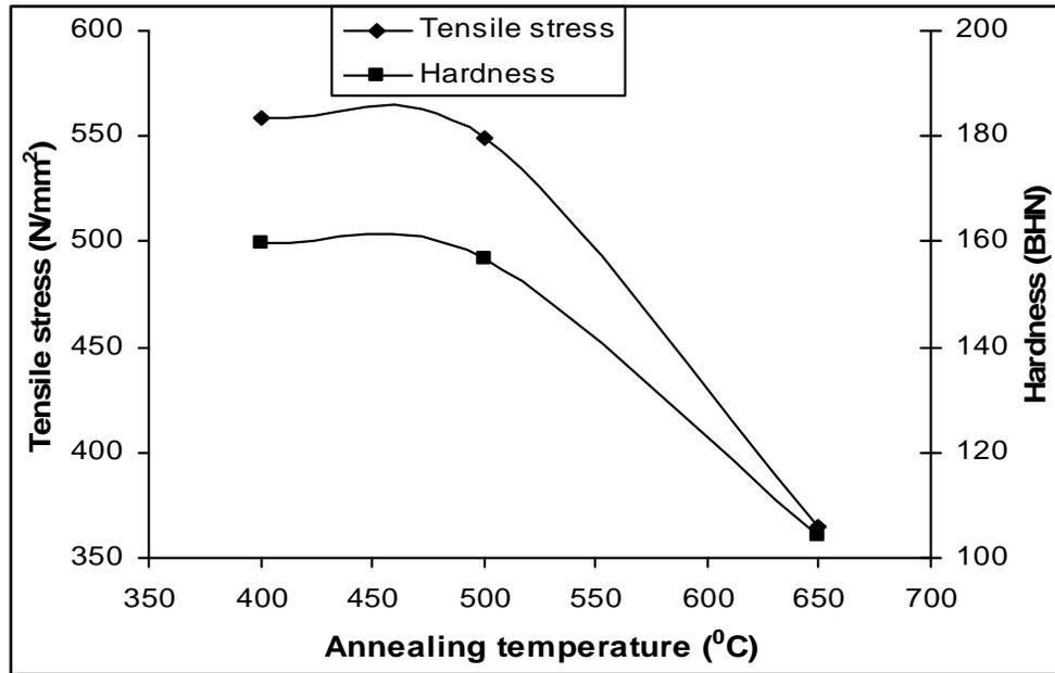
Fig. 3: Tensile stress and hardness versus annealing temperature
