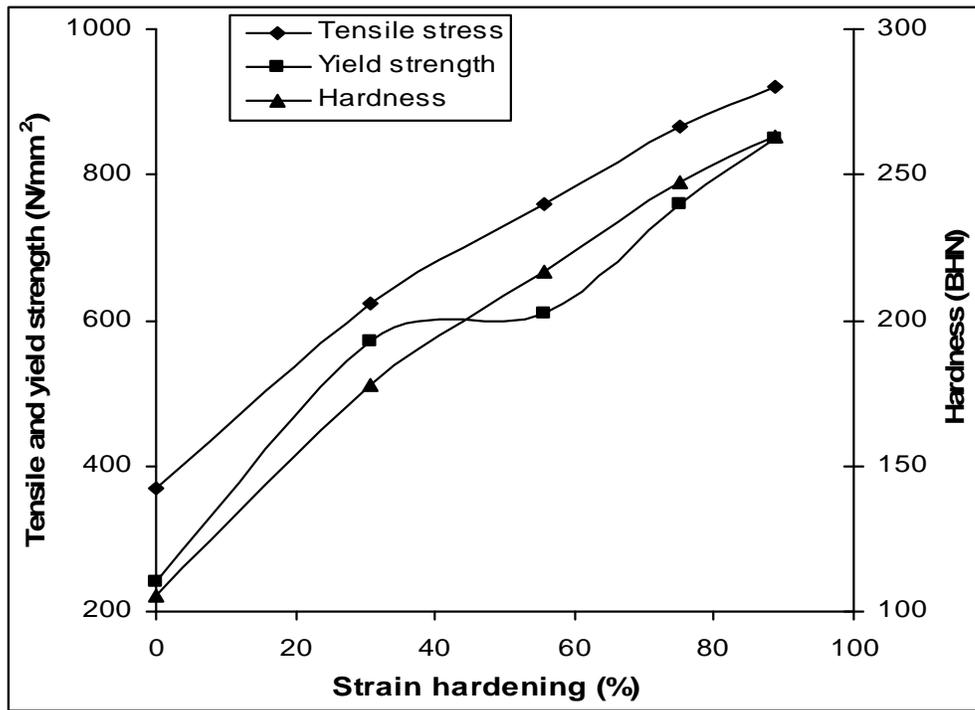
Fig. 1: Effects of strain hardening on the hardness and Strength of NS 34 LC Coiled Wire
