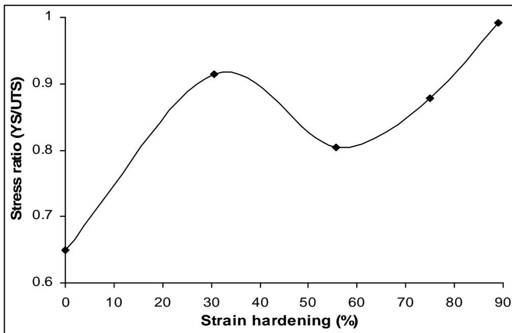
Fig. 2: Effect of strain hardening on the stress ratio (YS/UTS) of NS 34 LC Coiled Wire
