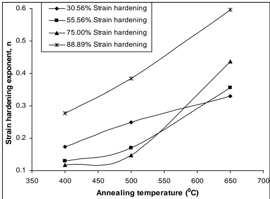
**Fig. 6: Effects of subcritical annealing on the strain hardening exponents, n, of NS 34 LC coiled wire**
