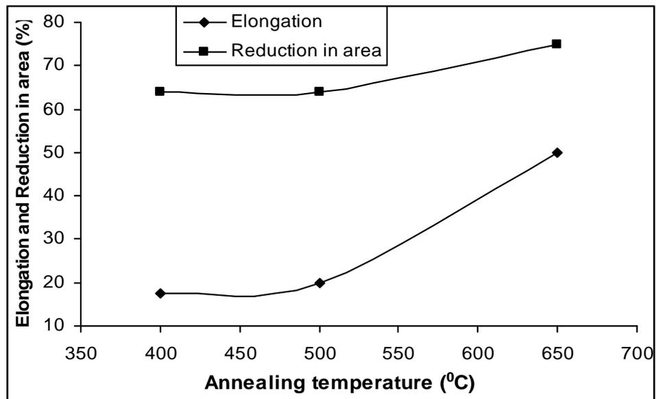
Fig. 4: Percentages of elongation and reduction in area versus annealing temperature
