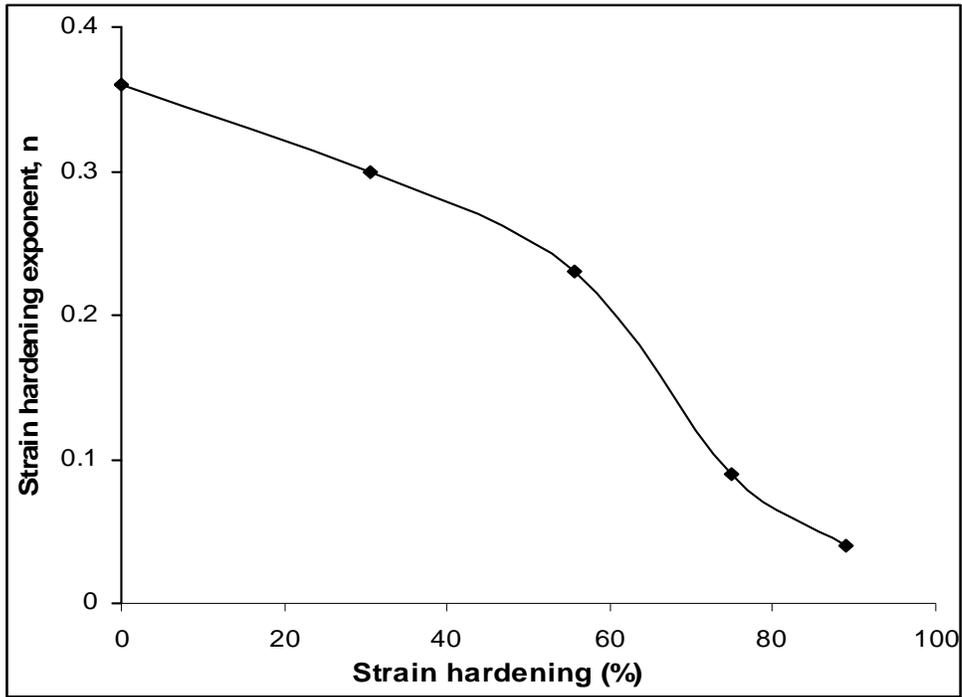
**Fig. 5: Effects of strain hardening on strain hardening exponents, n, of NS 34 LC**
