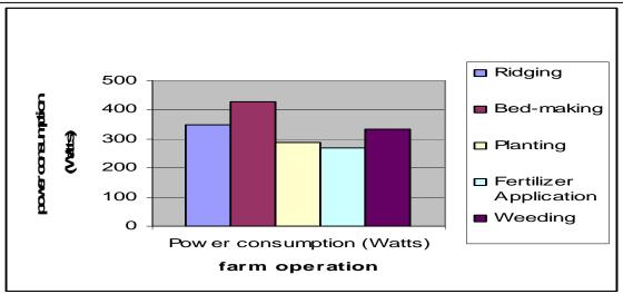
Figure 6: Mean power consumption against farm operation
