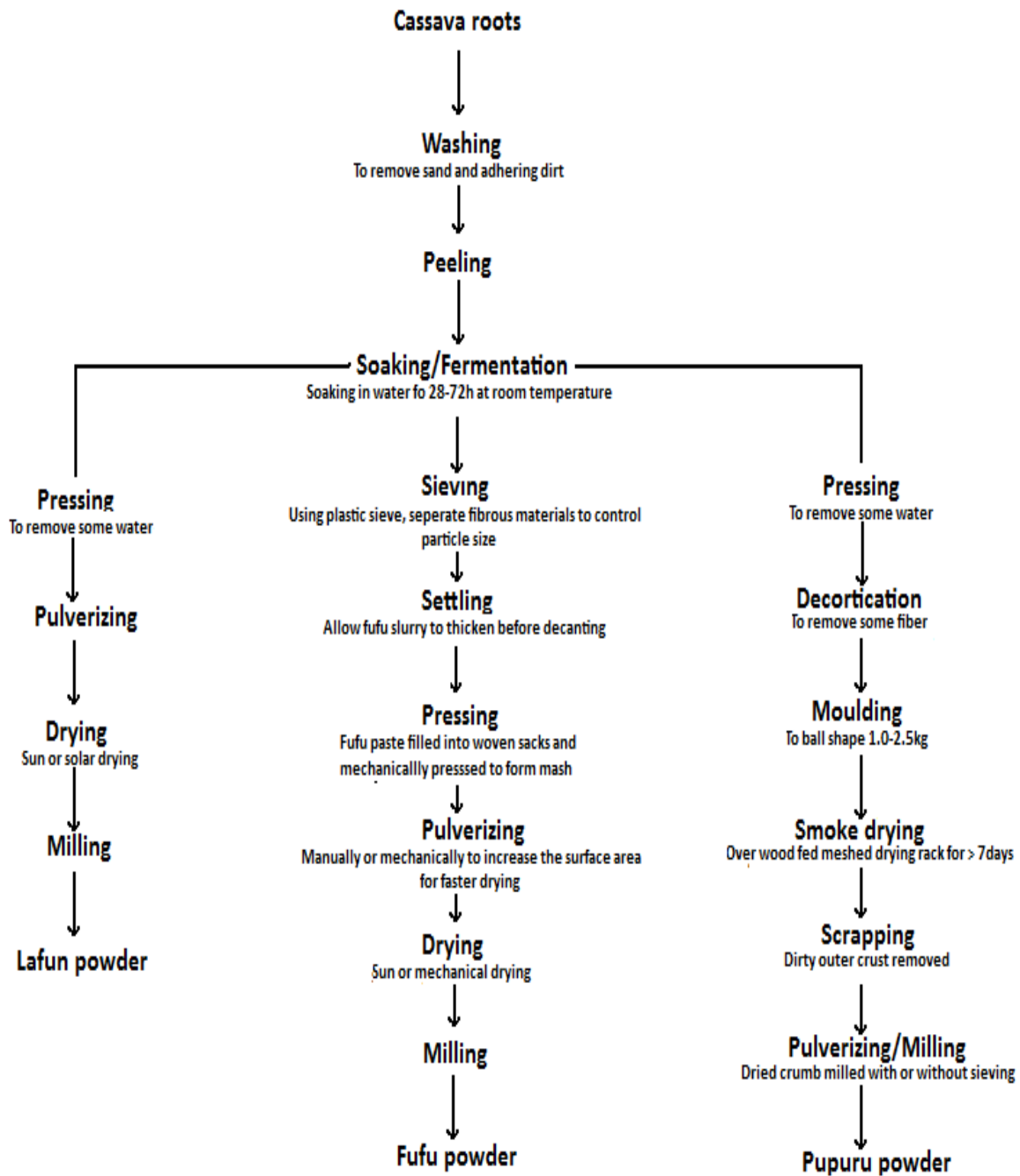
Figure 1: Chart showing traditional and/or improved steps followed in the manufacture of the fermented cassava products
