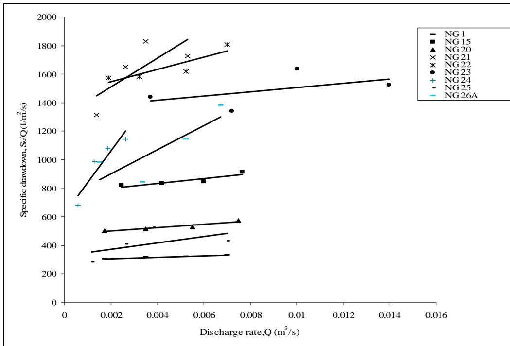
Figure 2: Plot of  $S_w/Q$  versus  $Q$  of field data from step - drawdown test
