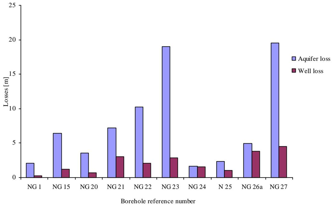
**Figure 4: Comparison of Aquifer and Well losses**
