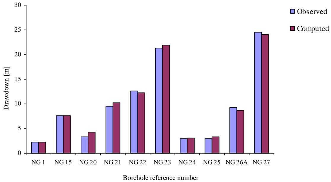
**Figure 3: Comparison of observed and computed drawdown**
